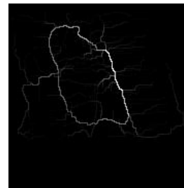
Figure 6. The edge confidence (EC) map formed by adding one to pixels where a shortest path goes through.
